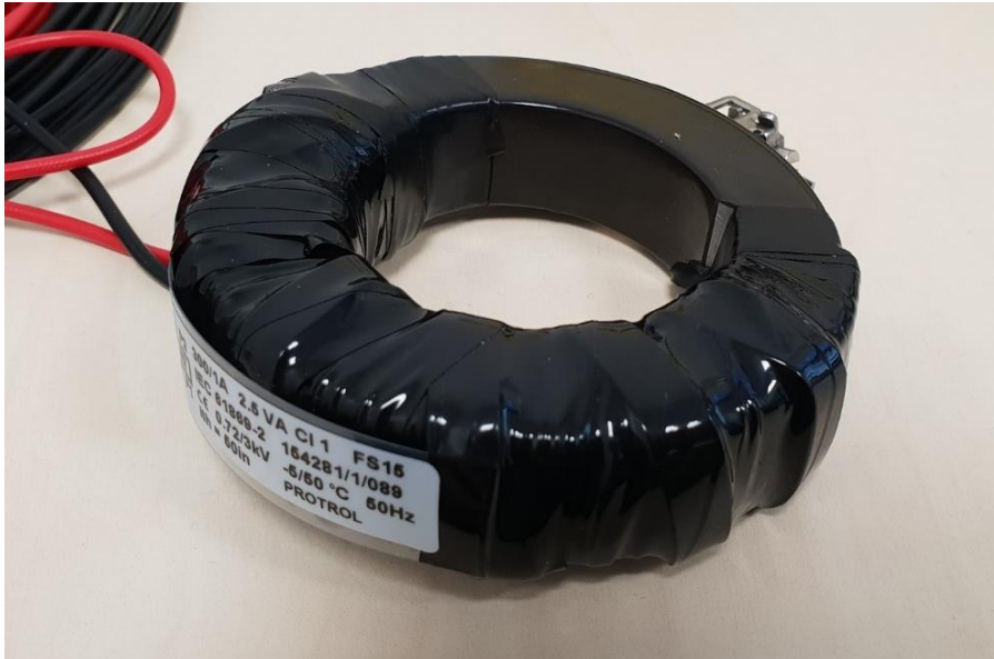
Figure 7: Split core current transformer of ring type with hose clamp for measuring current in a cable part.
