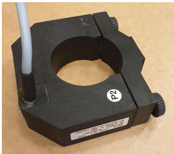
Figure 6: Split core current transformer with shielded cable measuring current in a cable part.
